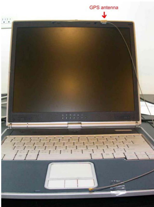
Fig 3-2. LS26050 with a GPS active antenna for a laptop.
